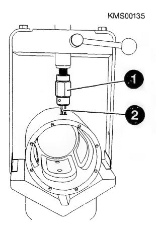
CHECKING AND REPAIRING COMPONENTS Replacing excitation winding Installation: Warm excitation windings before fitting, insert with pole shoes in stator frame and slightly tighten screws. Pay attention to markings. Press in driving-in mandrel. Driving-in mandrel diameter: 101,15 -0,05 mm
